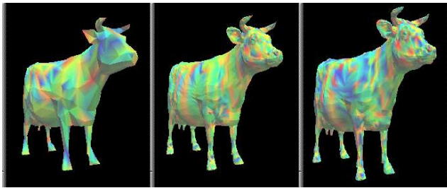
Fig. 8. Comparison images of multiresolution Cow object by comparing Gaussian curvature . Left and middle images are pseudo-colored using the Gaussian curvature. The image on the right is colormapped to the difference between the two sets of Gaussian curvature measurements.
