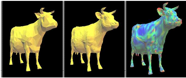
Fig. 7. Comparison images of multiresolution Cow object by comparing minimum distance . From left to right: coarse mesh, dense mesh, difference image using the rainbow colormap to locate the regions of high error.
