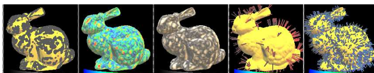
Fig. 6. Some visual mapping options for difference image. From left to right: overlay, rainbow mapping, white-black-white pseudo-coloring, glyph (hi-pass filter), glyph (low-pass filter).
