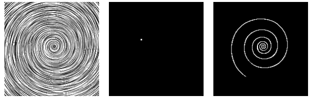
Figure 2: Left: Enhanced LIC image of the spiral data set. Middle: Input texture (only one pixel is turned on). Right: Result of repeatedly applying LIC to the input texture with only one pixel turned on.
